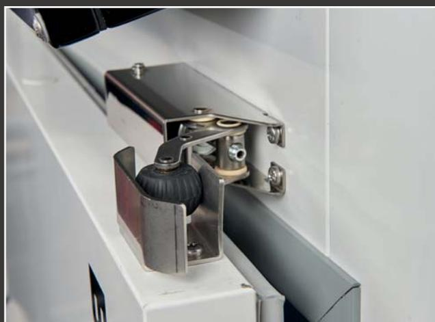
(2) detail of the hydraulic door-closing mechanism
